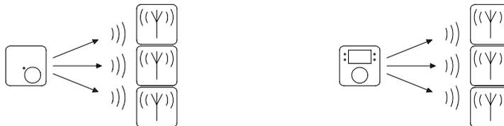
Averaging: (each receiver calculates the average value based on data from max. seven actual value transmitters and a transmitter with setpoint adjuster)
