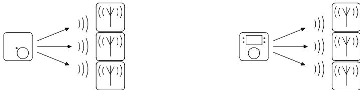
Averaging: (each receiver calculates the average value based on data from max. seven actual value transmitters and a transmitter with setpoint generator)
